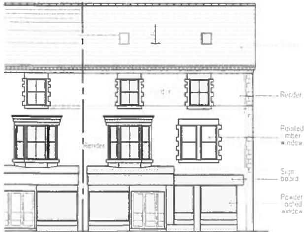
EXISTING FRONT ELEVATION
